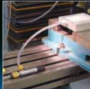
Vacuum chuck application: J-Series – vacuum holding for machine shop
