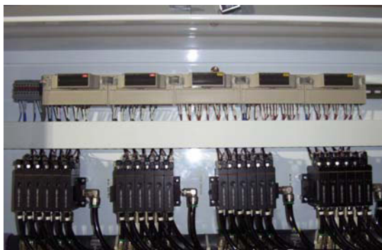
Flexible automation – Four, six station manifolds control an End-of-Arm Tool that configures different zones of cups to handle a wide variety of stamped metal parts. No tool change required.
